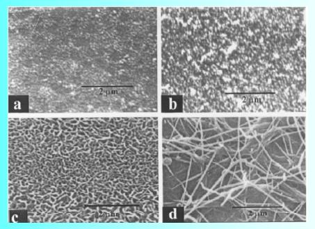
SEM microstructures of the films on tin-oxide coated glass deposited for (a) t=1 h (b) t=2 h (c) t=3 h and (d) t=4 h
